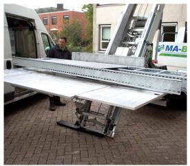
In addition, MA-BO offers Alu-cranes. Aluminum cranes are light (from 18 tons) and can also be used on difficult terrain or terrain that is difficult to access. Think, for example, of narrow access roads or bridges and access roads with a limited number of permitted tonnages. They have a maximum lifting capacity of 6 tons. The Alu-crane can be equipped with a 'fixed' work basket and is therefore a combination between a crane and aerial platform and therefore multi-usable.
